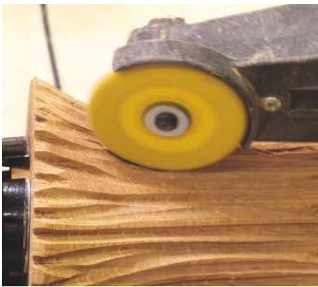
▲ Pic.10 The cutter is mounted in Les's Mini Arbortech grinder. This is the perfect tool for this job as it gives a really good finish in the grooves
